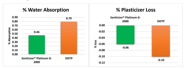
Santicizer® Platinum G-2000 Volatility (Carbon Method) shows the product to be superior to the DOTP tested. Tests were performed at 1 and 6 days and % plasticizer loss was recorded.
